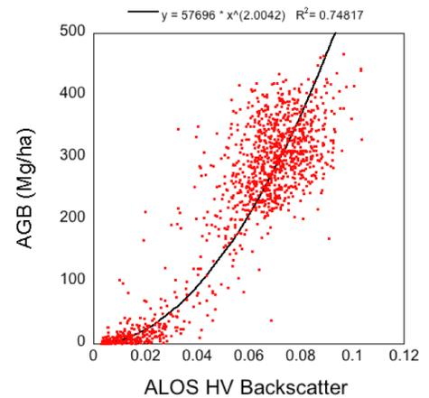
**Figure 1.8** An example of a best fit model between AGB and HV backscatter.
